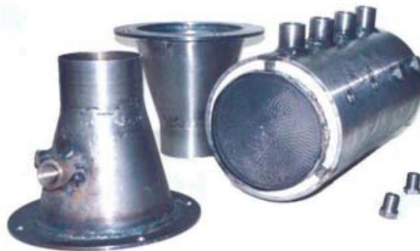
Fig. 12. Metallic enclosure of tested of catalytic converter [6]
